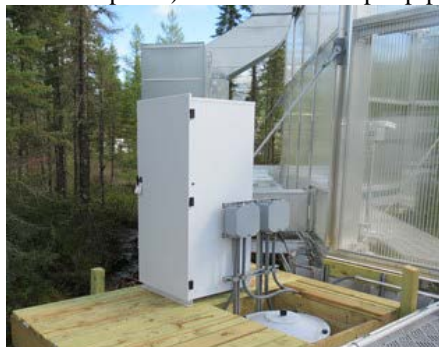
Photo (left) of a dock that surrounds and allows access to a sump basin (sump/enclosure 13). The photo also shows an autosampler, which houses a CR1000 datalogger/controller that measures the water level and operates the sump pump. Photo (right) showing the bottom of a large tank and the transitional rim (gray ring in right center of the photo) to the 15-cm deeper pipe.
