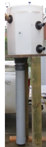
Photo (left) of a dock that surrounds and allows access to a sump basin (sump/enclosure 13). The photo also shows an autosampler, which houses a CR1000 datalogger/controller that measures the water level and operates the sump pump. Photo (right) showing the bottom of a large tank and the transitional rim (gray ring in right center of the photo) to the 15-cm deeper pipe.
